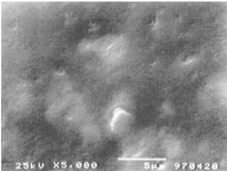
FIGURE 1 SEM Micrograph of the 90% Epoxy resin + 10% Hardener blend, cured by method 1.
